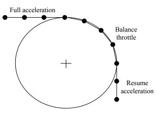
While accelerating in a straight line, the force produced by the engine (longitudinal acceleration) will often be less than the maximum frictional force. Exceptions to this might be a grid start, or a Formula One car running on cold tyres. It should therefore be possible to negotiate a corner whilst still accelerating.
