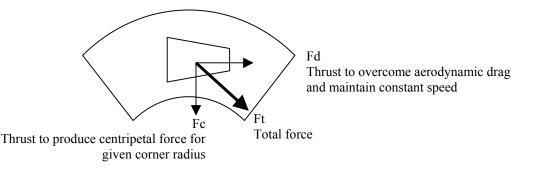
When the car is cornering at the maximum speed, the total force Ft will be equal to the maximum force that can be transmitted through the tyres:
