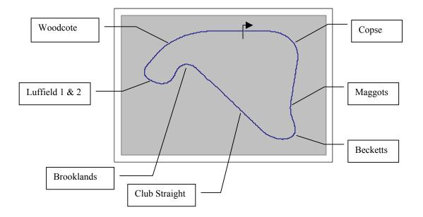
The circuit data from Silverstone contains corners whose radius reduces up to the apex, then increases as the driver tries to take the best line on the available track. It also contains corners where braking is required as the car is turning a corner (between Brooklands and Luffield 1).
