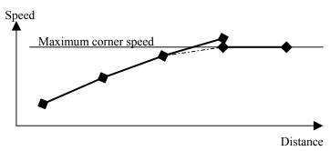
In reality, the driver would continue to accelerate until the maximum corner speed was reached, then hold that speed. As our track is split up into sectors, we can model this as shown in the diagram, where the exit speed is simply set to the maximum corner speed. The average acceleration will be the same regardless of how we model the transition, since the entry and exit speeds will be fixed.
