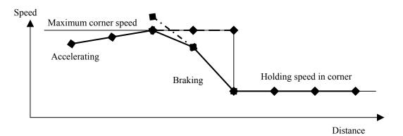
The initial calculation of maximum corner speed and forward acceleration can be done by progressing forwards through each sector in turn, feeding the exit velocity from one sector into the entry velocity of the next. To calculate the best possible braking performance, we will first calculate the acceleration from rest and maximum corner speeds, then apply the braking forces on a second pass, this time going backwards through the sectors.
