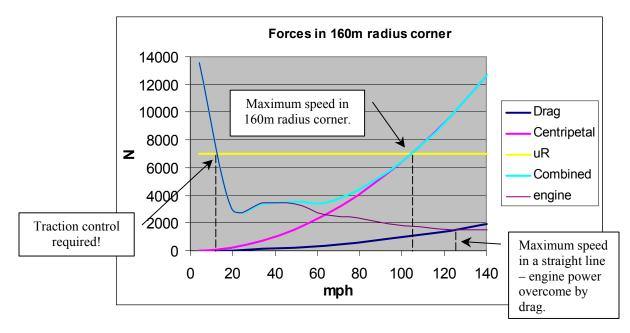
At slow speed, the available force from the engine would exceed the maximum frictional force and cause wheelspin if all the power was applied. At higher speed, it can be seen that the centripetal force becomes the dominating factor. The maximum speed is reached when the combined force is equal to the maximum frictional force. We can also see from the diagram that the maximum straight-line speed would be reached when the drag force becomes equal to the accelerative force from the engine.
