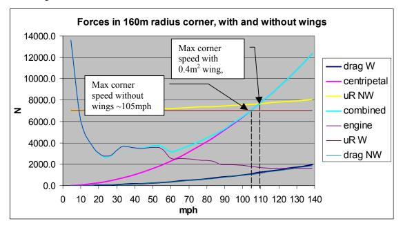
The wing will add extra drag to the car, again this is calculated using the coefficient of drag and the plan area of the wing:
