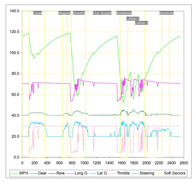
The plot below shows data from the model. It is in a slightly different form to the previous graph – this has been done to match the format of the data printed from the PI analysis software.
