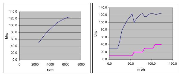
Again, this method could also be used given the torque curve of the engine. It is difficult to model the effect of gear change time using this method. When the engine is not accelerating the car, the car will slow down the revs will drop, and oscillation can occur on upshifts unless some hysteresis is introduced.
