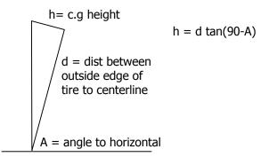
If the track were equal front and rear, the calculation would be very simple trigonometry.
