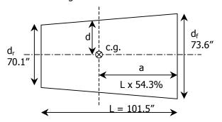
df = Between outside edges of front wheels: 73.6''dr = Between outside edges of rear wheels: 70.1''Wr = Weight on rear axle - 54.3%
