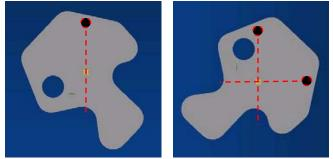
each point of suspension will reveal the c.g. at the point where the lines cross.
