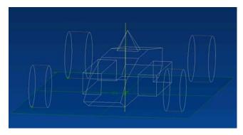
The approach chosen in this case was to balance the car on two points – the front and rear tire sidewalls of one side of the car. The vertical plane rising from these points must pass through the center of gravity.
