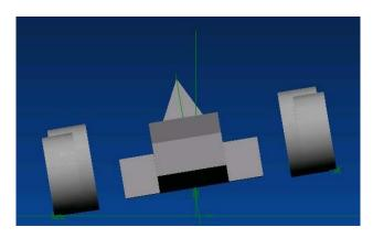
The theory goes that the center of gravity will be shifted towards the low side/end of the car, which will then weigh heavier. The height of the c.g. can then be worked out from the change in measured weights.
