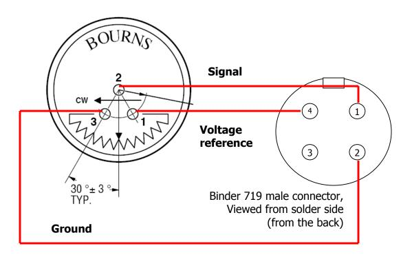
The above diagram shows a setup where the input voltage increases as the pot is turned in a clockwise direction.
