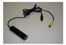
Camera and mic: Sony 580-line EX-VIEW, with 3.6mm lens, from <u>extremehelmetcams.com</u>
