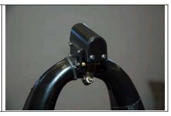
The picture above uses a mount from <u>helmetcamera.com</u>, with added side-plates to mount to the roll hoop.
